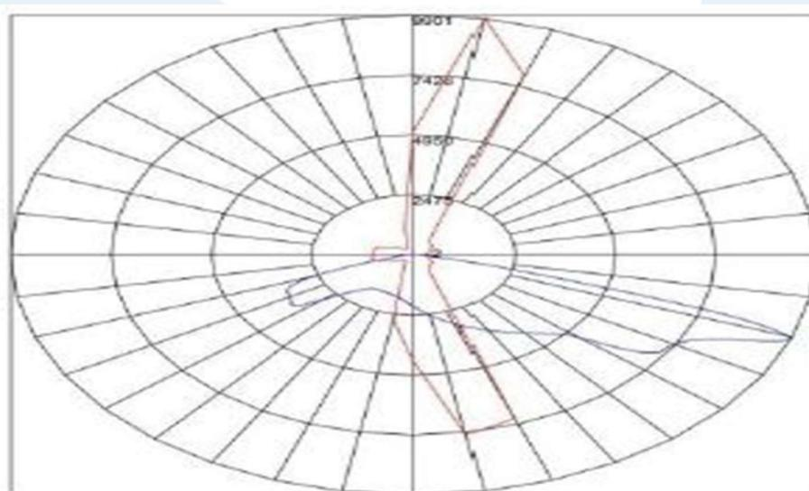
Maximum Candela = 9900.75 Located At Horizontal Angle = 80, Vertical Angle = 69.5
